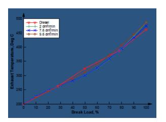
Comparision of exhaust gas temperatures between diesel and various hydrogen flows
