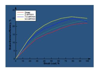
Break Thermal Efficiency as a function of Break Load for different hydrogen flow rates
